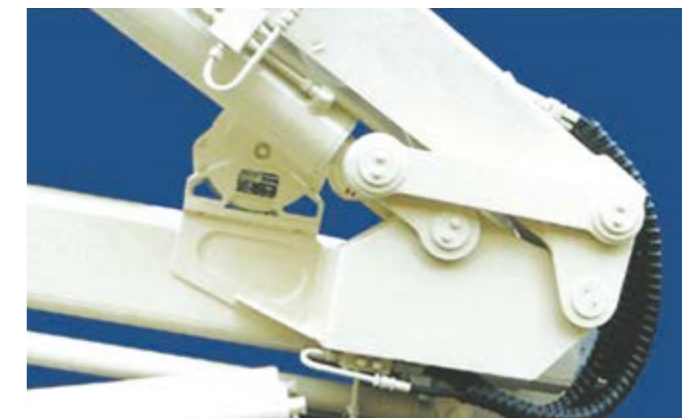
The link system of the outer boom gives additional power.
