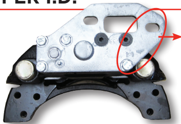
DX195 (6 bolt mount) Plate points right = 1A
