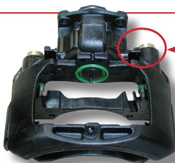
SAF Big slide pin on right viewed from inside axle = A
