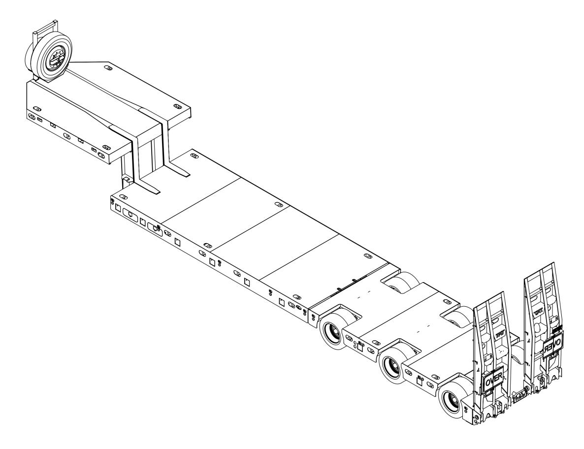
TOLERANCE : ± 0.5mm UNLESS OTHERWISE STATED WIRE BUFF ALL STEEL COMPONENTS PRIOR TO WELDING
